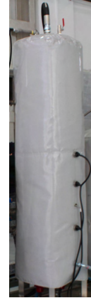
2 Bar 134°C Fully Automatic Steam Chamber
